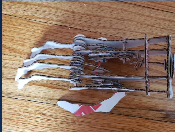
The hand with the thumb attached, and some of the gears associated with it. Certain gears for the center region have still yet to be attached.
