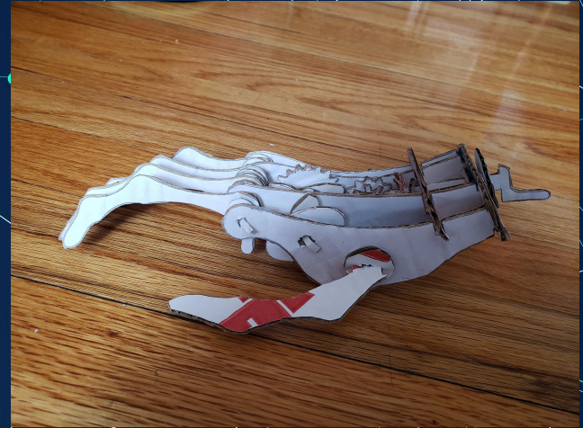
The finished hand. All the gears have been attached including the central ones, and the ones for the thumb.
