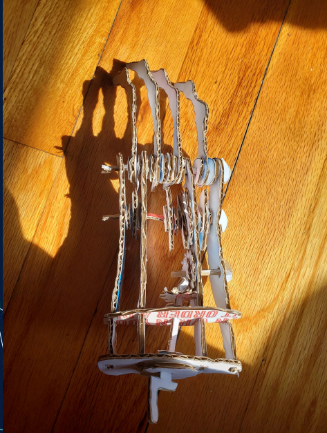
The hand with the four fingers attached, and individual support gears.
